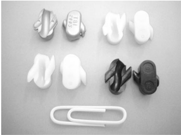
Figure 4 Photograph of ball-sliding parts made with S316 metal and nylon 66 compound.
