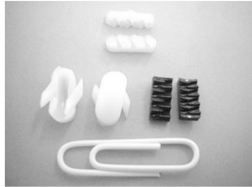
Figure 8 Photograph of ball-sliding plates with measured shrinkage.
